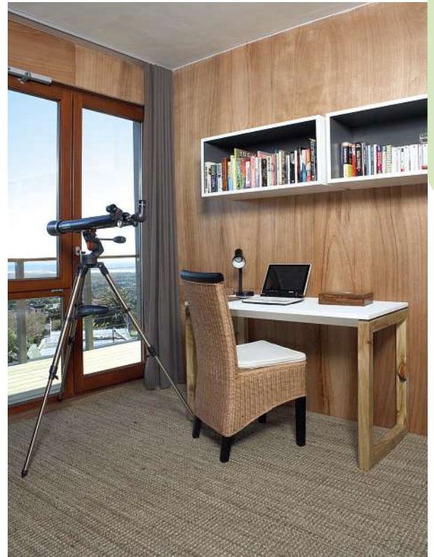
Tony's study (above) have hemp particle boards veneered with a thin layer of wood on the walls, ideal for insulation. The bath (below) is clad in bamboo, enhanced by water-saving fittings from Hansgrohe.
